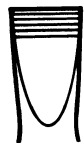
Ribbed: The interlocking teeth of the ribbed system provide higher torque. Components in the system are interchangeable with standard Slotted components.
