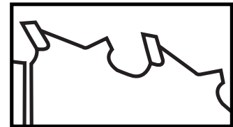
Strengthened shoulder adds strength behind the tooth and prevents overfeeding.
